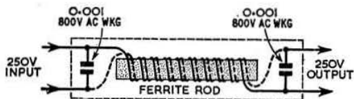
Fig 4. Bifilar mains choke wound on a transistor radio ferrite rod. About 30 double turns of adequately-rated pvc-covered wire closewound on a 1/2 in diameter rod should suffice (dimensions and turns not critical)
